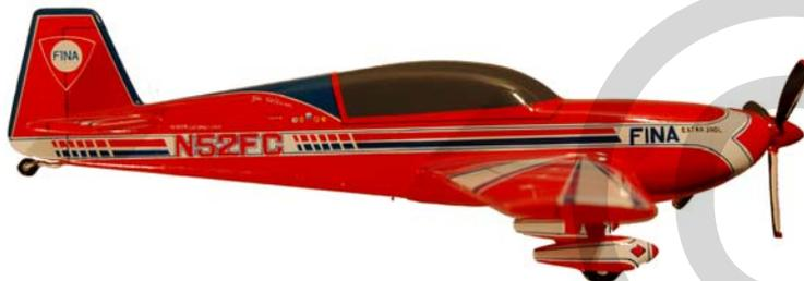
The **Extra 300L**, which we have used as a model in the following pages, competes in the unlimited category and is approved to plus/minus 10G's, has a roll rate of up to 400° per second and will cruise at 170 knots. It has two seats in a tandem arrangement, fixed landing gear, a constant speed propeller, and a six cylinder 300 HP engine. And, it is a great looking airplane!
